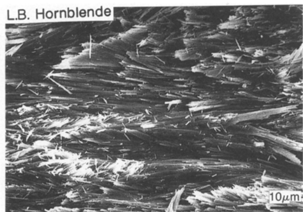
Figure 10 Fracture surface of LB hornblende showing much more pronounced fibrous nature and high degree alignment of the fibres.
